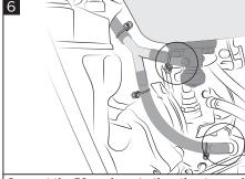
Connect the 30mm hose to the other tap and the remaining one to the carburetor as shown in the figure.
