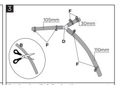
Cut the pipe (B) following the measurements shown in the figure and connect it through the Y fitting (D). Fit the hose clamps (F). Tagliare il tubo (B) seguendo le misure indicate in figura e collegarlo tramite il raccordo a Y (D). Calzare le fascette stringitubo (F).
