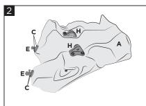
Fit the original connections (H) and the taps (E) using the screws (C).
