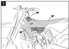
Remove the spoilers and the saddle and disassemble the original tank.
