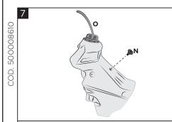
Assemble the original tube (O) in the cap. Tighten the original saddle screw (N).
